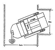
Aisle dimensions listed above assume the minimum bay width to be straddle OD plus 5° (2.5° on each either side of straddle log). Straddle OD is the load width plus 8°. Truck performance may vary due to application requirements' and changes in model design.
